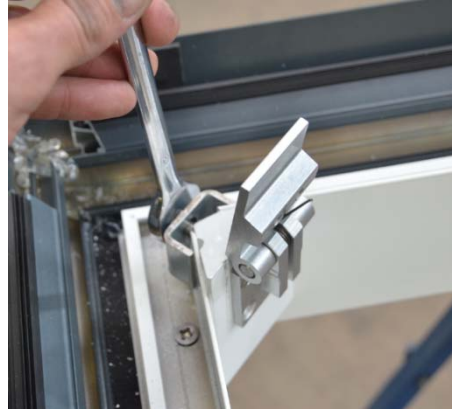
Position corner block & tight bolt.
