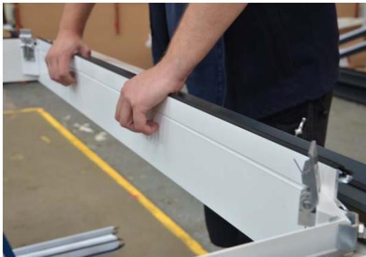
Push in large eaves clip, start in corner & place bar bracket in between eaves clip to set out bar positions.
